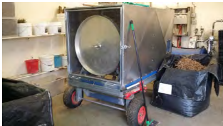
The seed tumbler used to more effectively separate seed and chaff
