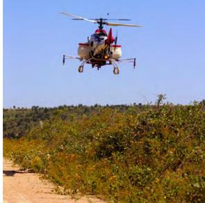
Low spray height and rotor down wash minimises off-target damage. Part of a virtual tour viewpoint below shows the RMAX achieved a good kill on the blackberry using triclopyr herbicide, without damaging the Cassinia shrubs.
